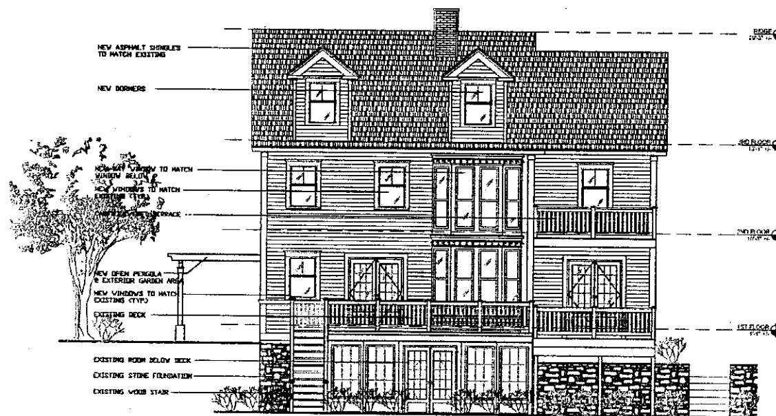
5 PROPOSED EAST ELEVATION SCALE: \frac{1}{8}'' = 1'-0''
